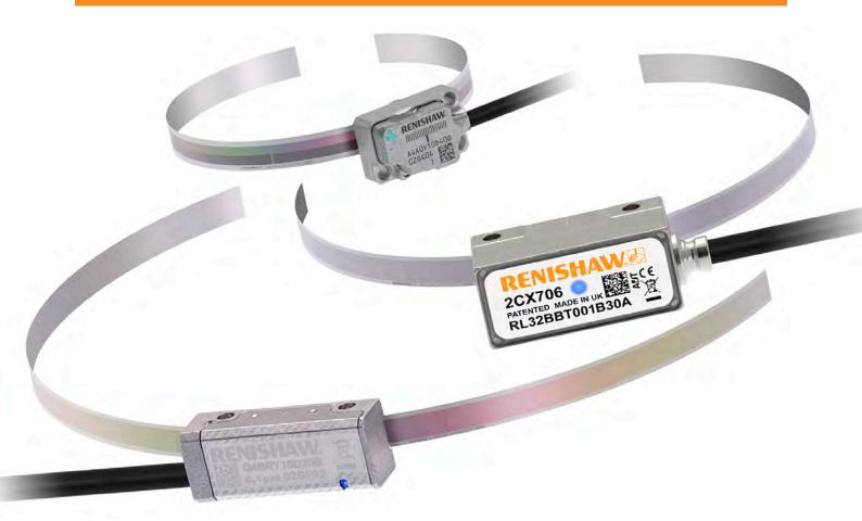
Measuring a partial arc of rotation is made easy with Renishaw's flexible RKL encoder scales. The flexible nature of the small cross-sectional area of these scales allows them to be wrapped around a drum, shaft or arc with a minimum radius of 26 mm.
