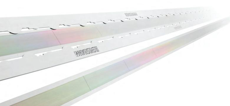
RTLC 20 or 40 µm linear encoder tape scale combines ±5 µm/m accuracy with the ruggedness of stainless steel. Two versions are available: self-adhesive RTLC-S and RTLC for use with the revolutionary *FASTRACK*™ track system from Renishaw.
