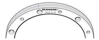
*IN-TRAC* reference mark is embedded in the scale, radially aligned with the centre of the mounting hole to the left of the 'Renishaw' logo, within ±0.5 mm. No external actuators or physical adjustment are required.
